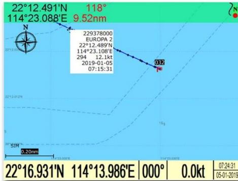
Points in the track shows the location, date, time, SOG and COG, etc.
